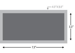
Rectangular Bar Metal weight savings: 25% compared to standard 4" x 8"
